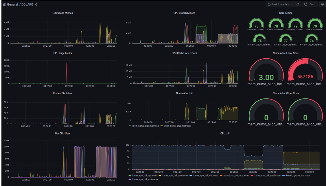
Figure 3 An example Grafana dashboard showing performance metrics collected by PCP and indexed with InfluxDB on a single host. Exhibiting node-level monitoring usage.
