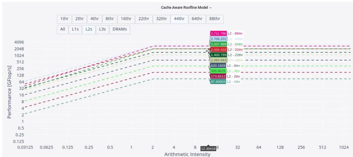
Figure 7 Roofline dashboard model generated with plotly is interactive and allows selecting data. In this figure, peak performance of L2 caches with different multi-threading settings is selected.
