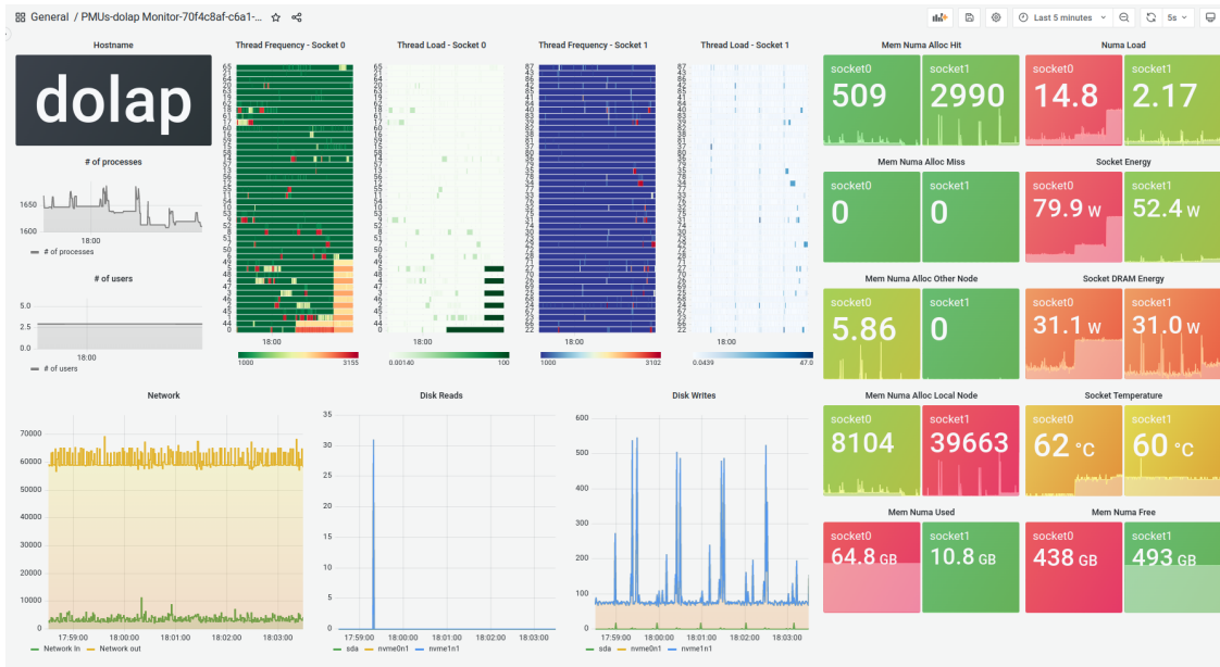
Figure 9 A live monitoring dashboard that is tailored for machines that have multiple NUMA domains. As mentioned, metrics are paired with panels that match their value type and meaning best. Since topology information is also captured by STD, rows in thread load and thread frequency panels are sorted w.r.to shared cores automatically. This way, events that effect topologically close threads could be observed more clearly. For example, in this dashboard a load is placed in threads 0, 1, 2, 3, 4, 5, however frequency is also increased in threads that share core with this threads. Since the JSON object that translate into this dashboard is mutable, new metrics with desired panel type could be appended by user at any time.
