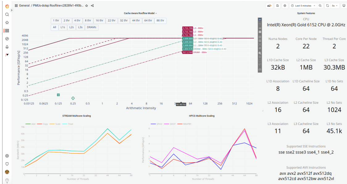
Figure 6 A roofline dashboard with combined results of CARM, STREAM, HPCG and system specifications. As mentioned, benchmark results are stored as BenchmarkInterface in the twin description. Note that, because the metrics required to calculate Arithmetic Intensity of an execution is collected during the execution of benchmarks, STREAM and HPCG benchmarks are marked on the roofline. Storing benchmark results in STD allows re-generation of the roofline model and mark the executed application if required metrics are collected. Instability in STREAM and HPCG benchmark's results are due to incomplete NUMA placement module.
