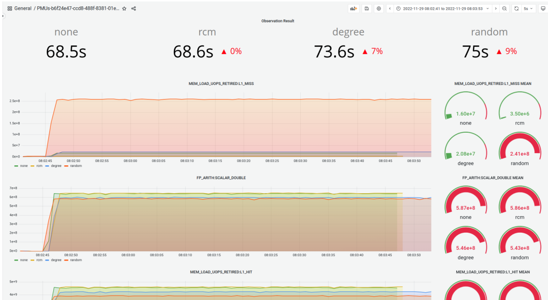
Figure 11 A comparison dashboard generated using four ObservationInterface that belong to the same system. In this figure, same SpMV kernel that use different orderings are compared. Collected metrics are originally from different times but their timestamps are synchronized in order to be able to observe program phases. This method will further developed with the addition of annotations that highlight program phases.
