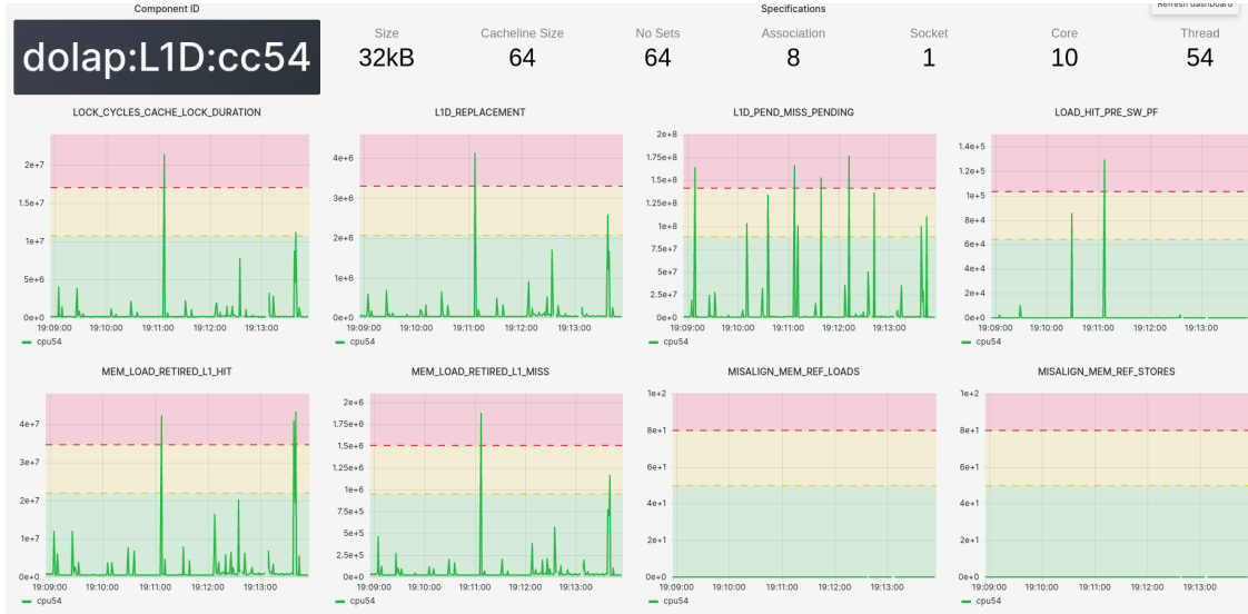
Figure 10 A component dashboard that is generated for L1D cache on thread54. As mentioned, Interfaces that make STD could be isolated from each other and could be used to generate exclusive dashboards for the component. Dashboards for network, disks, sockets, cores, threads, L1, L2, L3 caches are generated automatically via filtering the metrics that the system report at the time. When the metrics collected from the system change, panels on these dashboards are also automatically changed. Specifications panel on this dashboard is generated with embedding Plotly indicators that shows static information that is encoded in STD. Also note that visualized metrics on this dashboard are PMU metrics that are normally collected when an execution takes place. However, they are set to be monitored constantly therefore provide a live view on the component.
