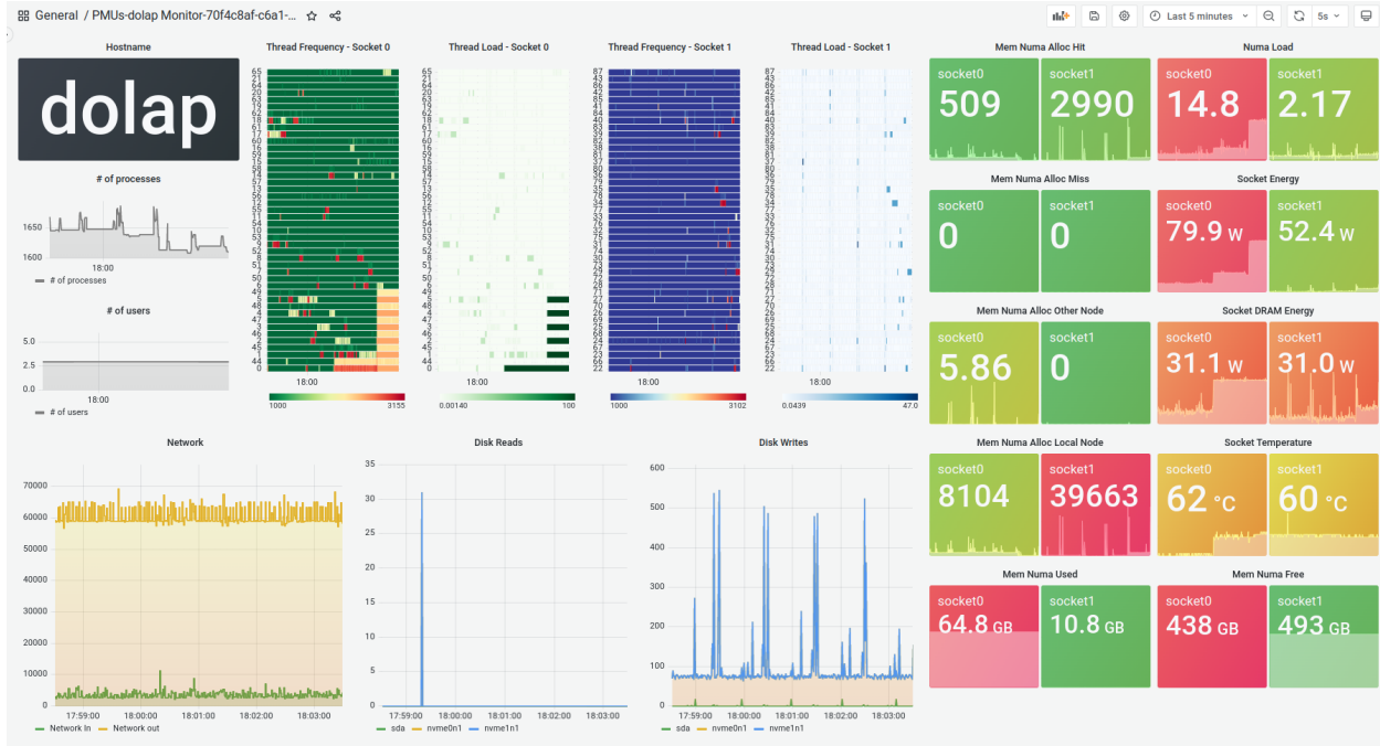
Figure 78 Generated Monitor dashboard for host Dolap. In the socket panels, threads sharing the same L1 cache are plotted consecutively, leveraging STD. At the time of the screenshot, a computation that is just launched in NUMA socket 0 but anomalously allocates memory from NUMA socket 1.
