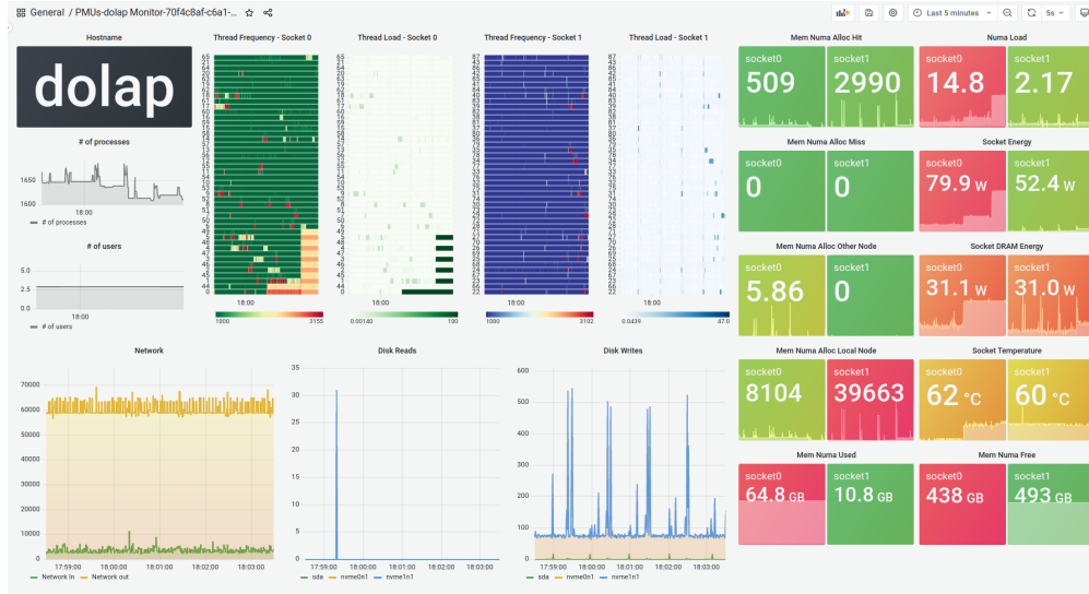
Figure 13 The Monitor dashboard for a single-node host Dolap. In the socket panels, threads sharing the same L1 cache are plotted consecutively, leveraging STD. At the time of the screenshot, a computation that is just launched in NUMA socket 0 but anomalously allocates memory from NUMA socket 1. This dashboard is accessible via link in Figure 10 and configurable by choosing metrics as in Figure 11.
